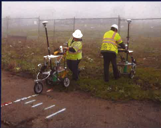
Workers perform a gamma walkover survey at Site 33
