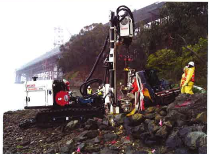
A sonic drill rig is used to collect boring samples at YF3
