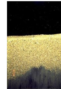
Thin-layer capping of contaminated sediment
