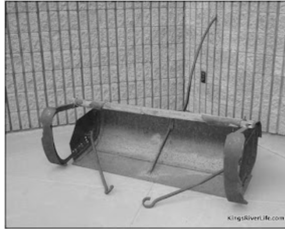
Fresno Scraper, invented by James Porteous, 1883
