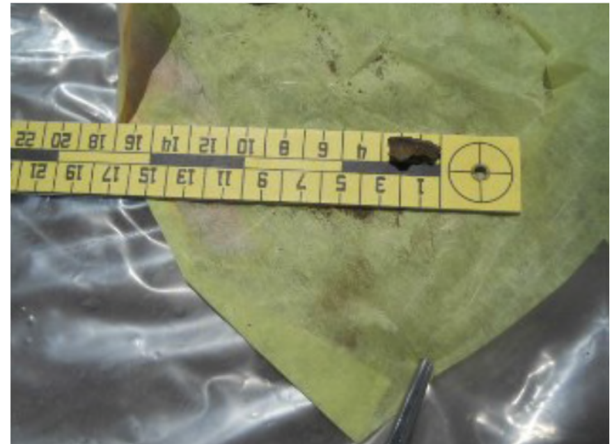
July 30 (metal fragment) –origin Excavation Area L2. Dose reading with NaI detector was 10 uR/hr at 12 inches
