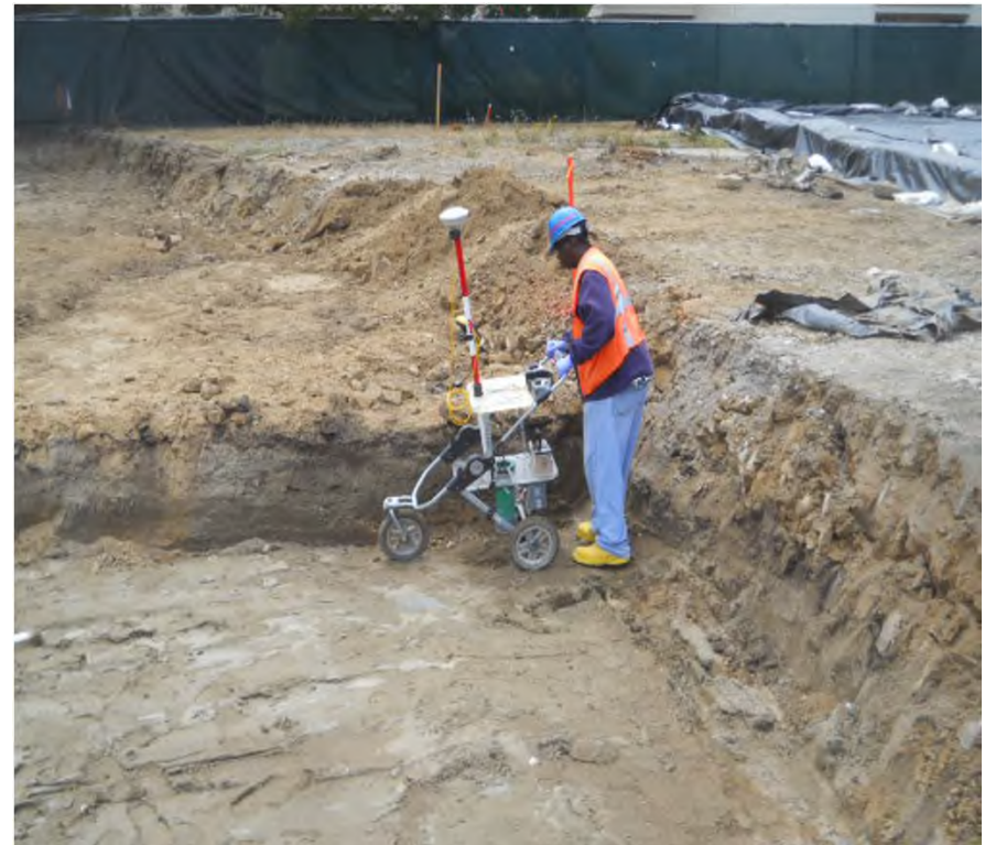
Gamma survey in Excavation Area D
