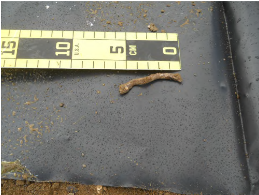
July 21 (copper pipe segment) – origin Excavation Area E. Dose reading with NaI detector was 26 uR/hr at 12 inches
