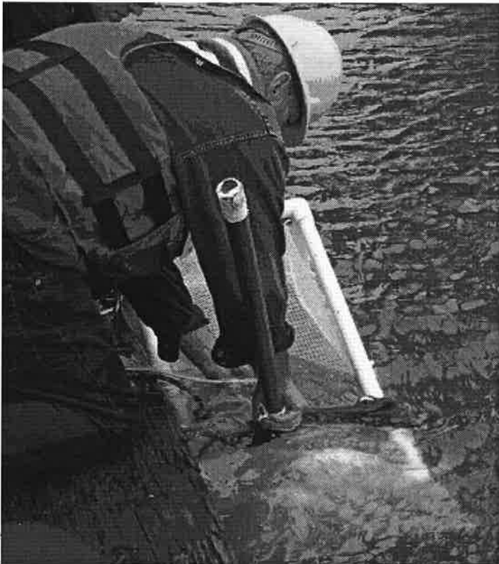
Figure 9. Cage with the hydrophone inserted through the mesh at the top end of the cage
